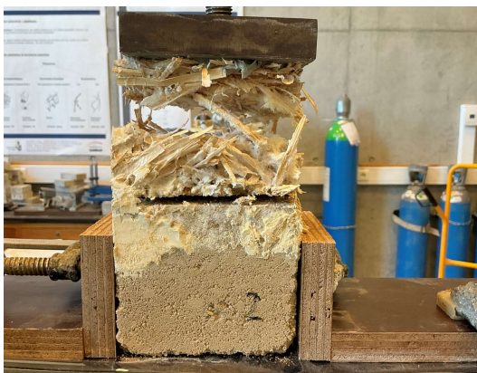
Figure 64 - Rupture de COM-PO-EN-P-2
